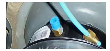
Caution: Release compressed air line connection slowly, compressed air flows out! Do not kink, twist or squeeze the compressed air line.
